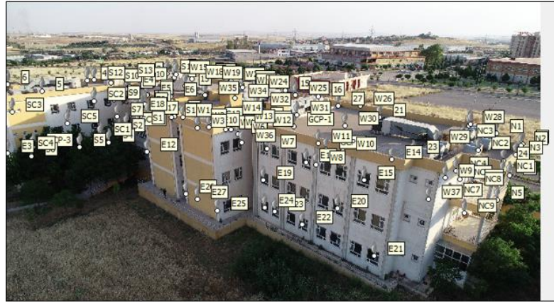
Figure 17: Revealing all sides of the control points: The East side, the West, and South facades
