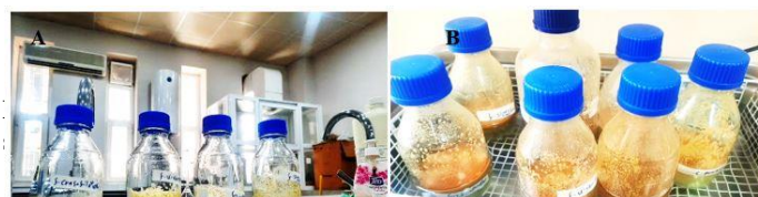
Figure 3: Main steps of bulb extract of Fritillaria spp. (A) alkalized sample with ammonia, (B) samples' incubation in ultrasonic bath, (C) samples after filtration, and (D) residues dissolved in 20 ml methanol.
