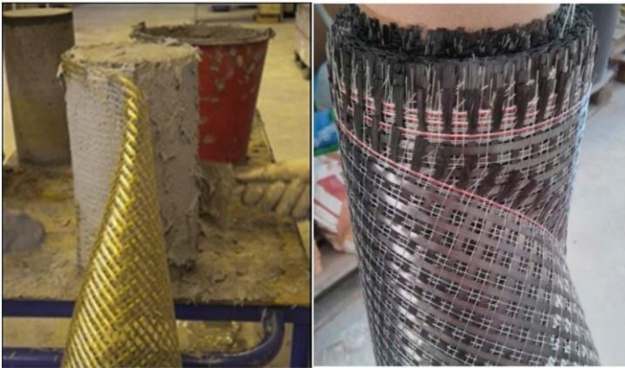
Figure 1: Application of fabric impregnated by cementitious matrix [9] .
