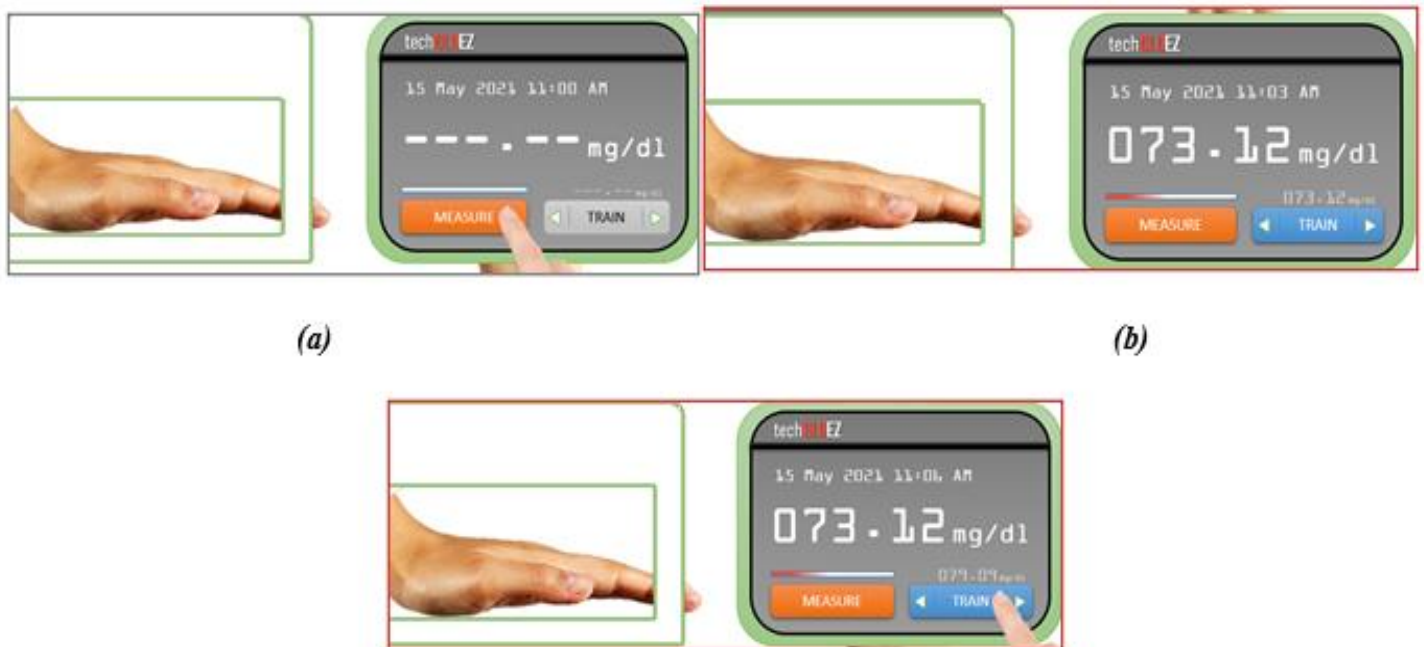
(a) Slide in Left palm and Measure Glucose level (b) Glucose level is displayed in 2-3 Sec (c) Train Glucometer for accurate results.
