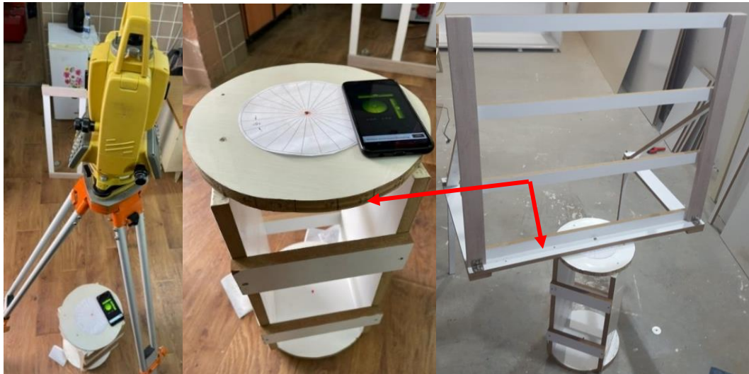
Figure 3: Test the verticality of the stand using the centering vertical laser beam of the total station instrument, two right photos for verticality test, and left image shows the controlling scan angle
