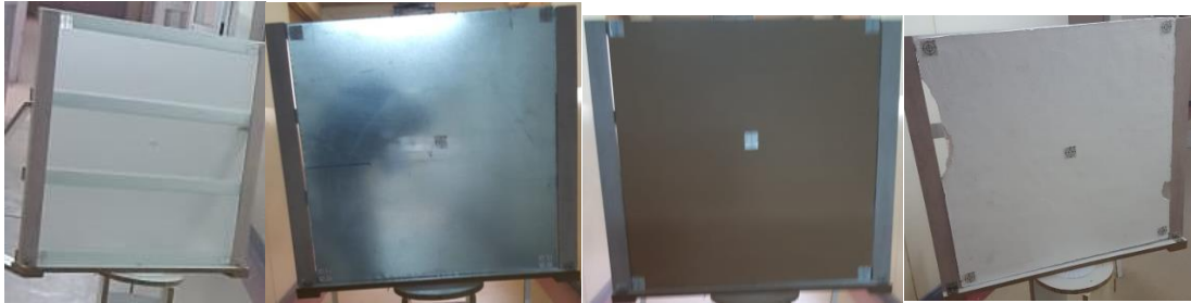
Figure 1: All materials used for scanning in different angles using ScanStation2 materials from left to right are Glass, Steel, Wood, and Ekoplast
