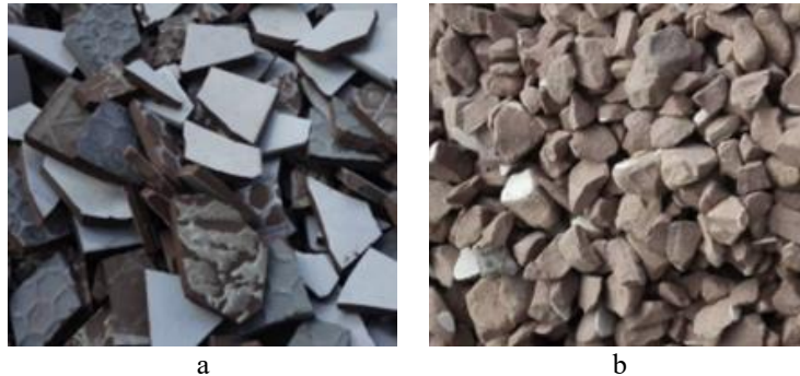
Figure 3: Coarse ceramic tiles a) Locally obtained waste ceramic, b) Crushing waste ceramic.
