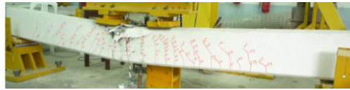
Figure 14. Failure mode of strengthened (PSC) beam with NSM reported by Obaydullah et al (2016) [94] .
