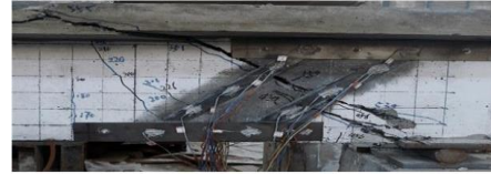
b) strengthened (PSC) beam with inclined strips
