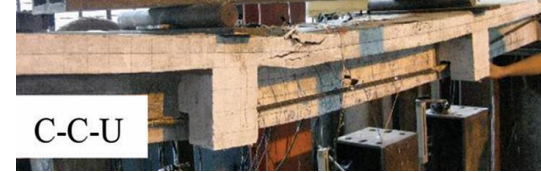
d) Strengthened (PSC) beam by external (CFRP) tendon (C-C-U)
