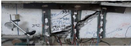
a) strengthened (PSC) beam with vertical strips
