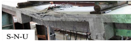
a) (PSC) beam with internal Steel tendon (S-N-U)
