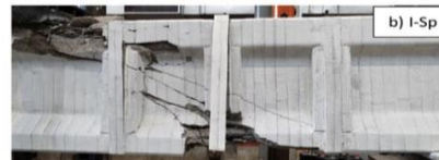
b) Shear strengthening system with (Fe-SMA) strips
